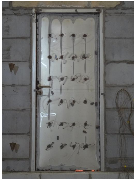
Fig. 10 Unexposed Side after 80 Minutes
