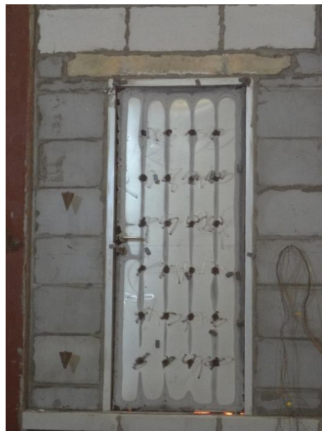
Fig. 14 Unexposed Side after 120 Minutes
