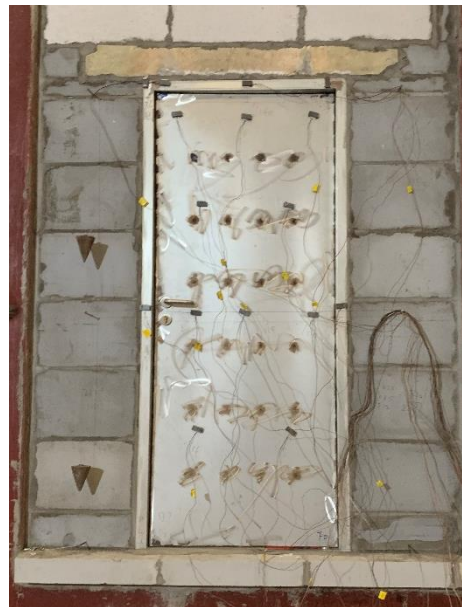
Fig. 4 Unexposed Side after 20 Minutes
