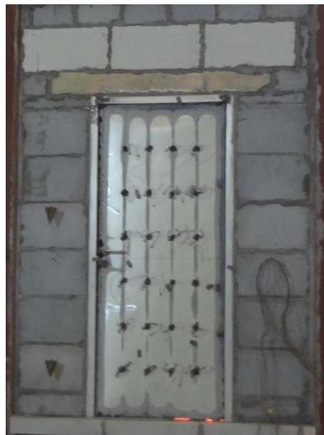
Fig. 12 Unexposed Side after 100 Minutes
