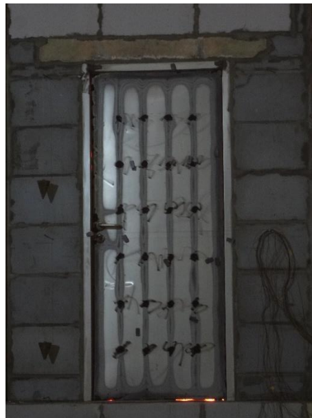
Fig. 20 Unexposed Side after 180 Minutes
