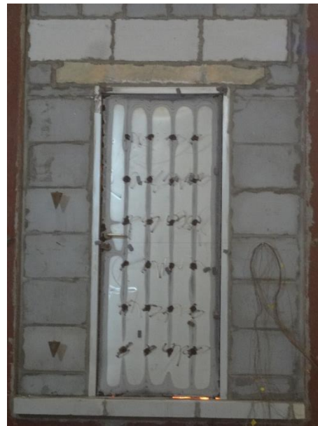
Fig. 16 Unexposed Side after 140 Minutes
