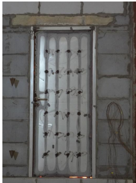
Fig. 18 Unexposed Side after 160 Minutes
