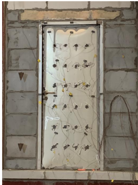
Fig. 8 Unexposed Side after 60 Minutes
