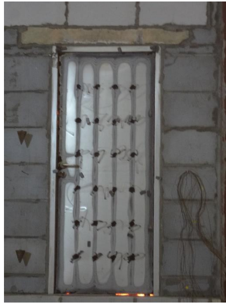
Fig. 19 Unexposed Side after 170 Minutes
