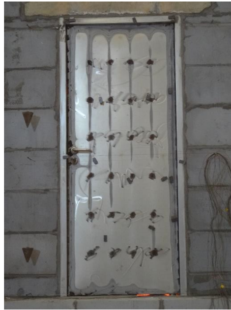
Fig. 11 Unexposed Side after 90 Minutes
