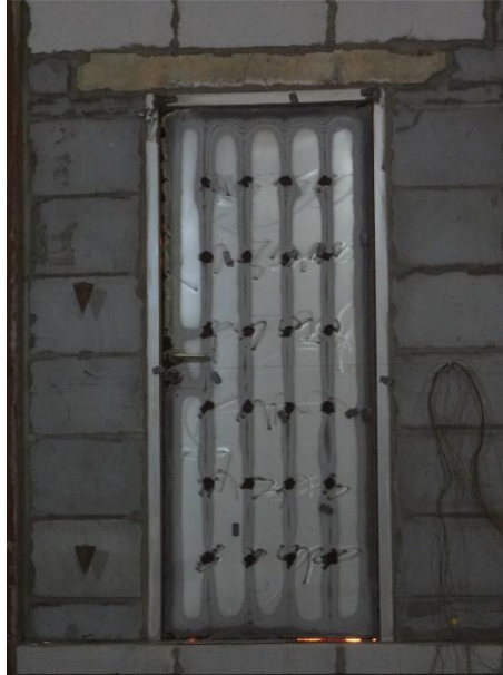
Fig. 23 Unexposed Side after 220 Minutes
