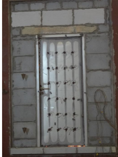
Fig. 17 Unexposed Side after 150 Minutes
