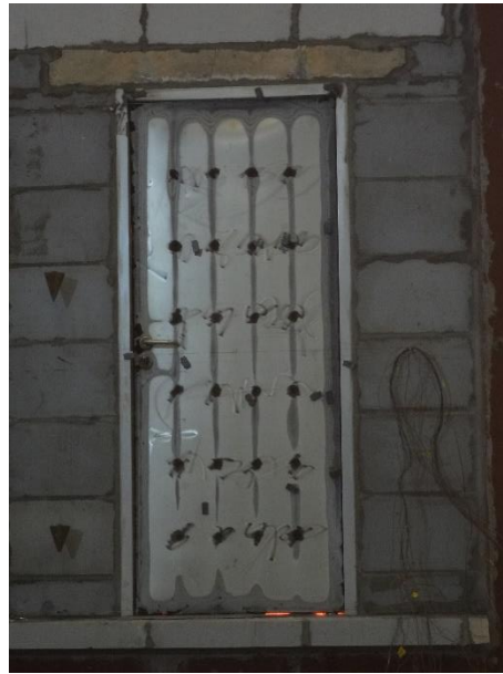
Fig. 13 Unexposed Side after 110 Minutes
