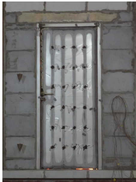
Fig. 22 Unexposed Side after 200 Minutes
