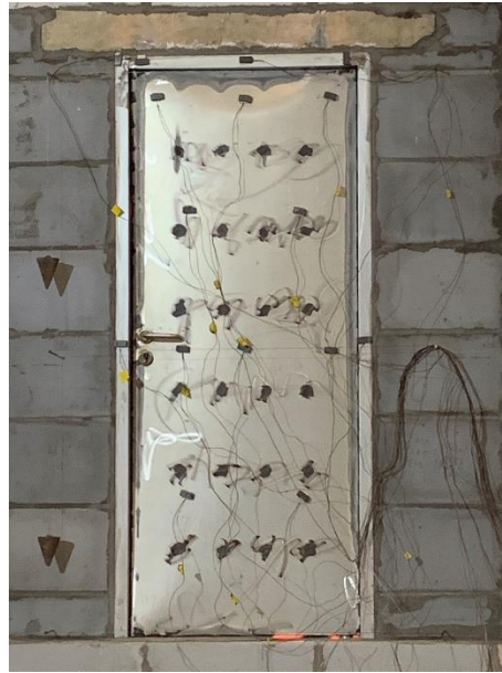
Fig. 7 Unexposed Side after 50 Minutes
