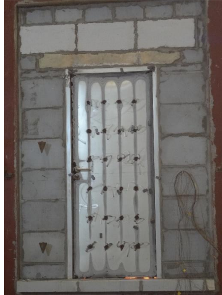
Fig. 15 Unexposed Side after 130 Minutes
