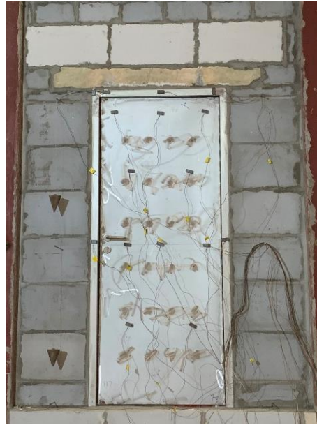
Fig. 3 Unexposed Side after 10 Minutes
