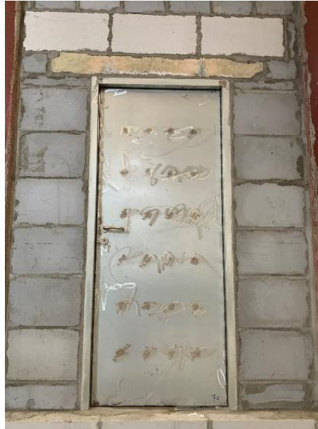
Fig. 1 Unexposed Side Prior to the Fire Test
