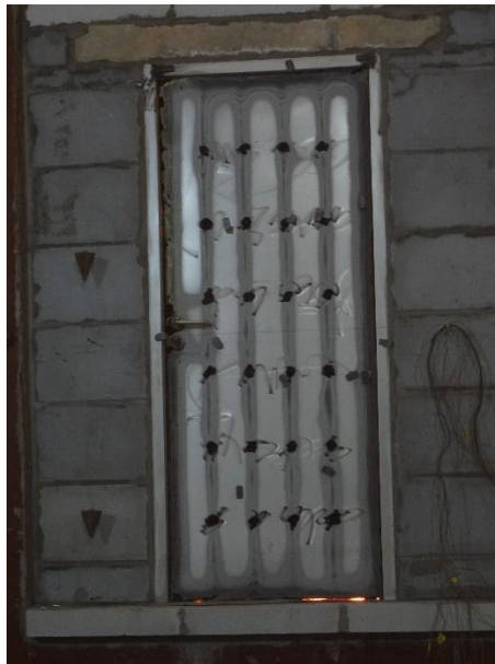
Fig. 24 Unexposed Side after 240 Minutes
