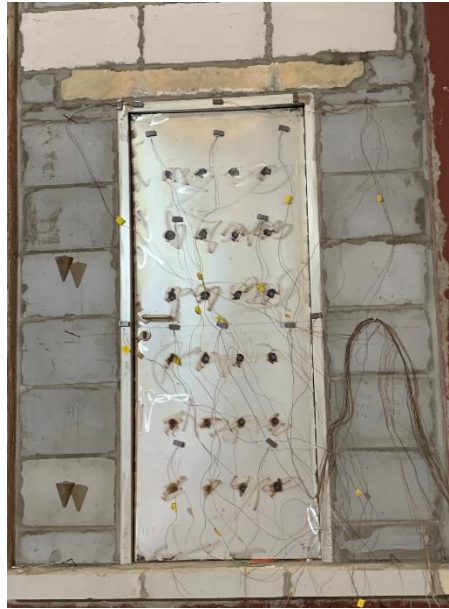
Fig. 5 Unexposed Side after 30 Minutes
